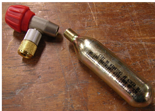
Figure 10: A 16g disposable cylinder of liquid carbon dioxide, of the type used for this project, and a fitting to attach it to a bicycle tyre. The fitting pierces a seal on the stem of the cartridge when screwed on.
