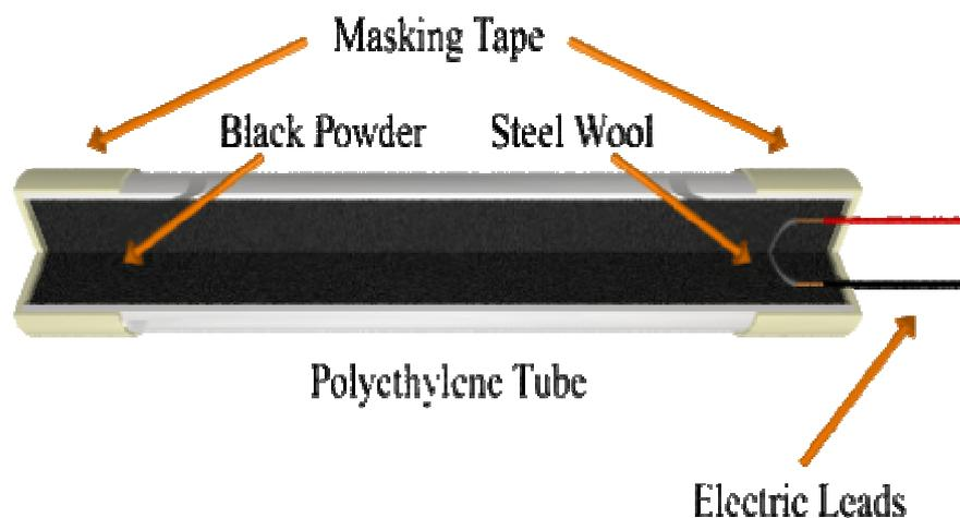
Figure 3: Rocket Ignition Device
