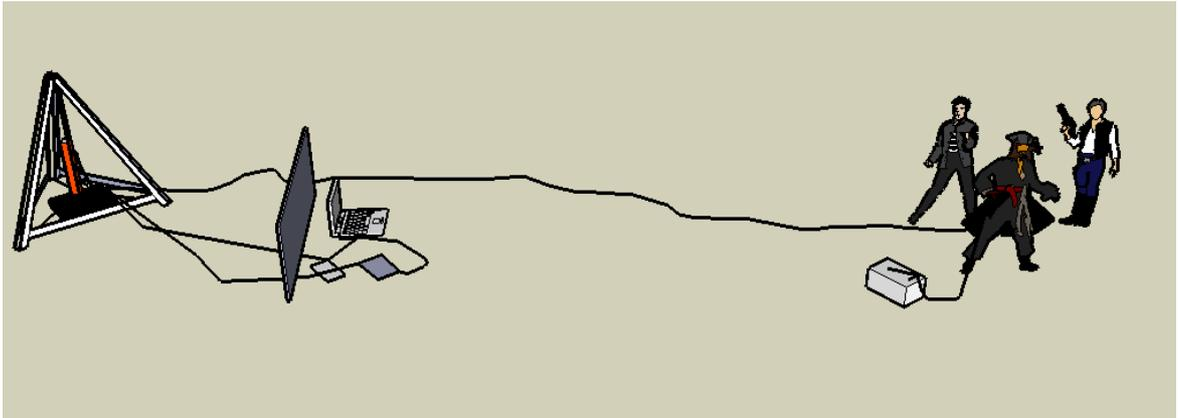
Figure 8: A distance of at least thirty feet between the experimenters and the rocket is shown, as is the ignition device.
