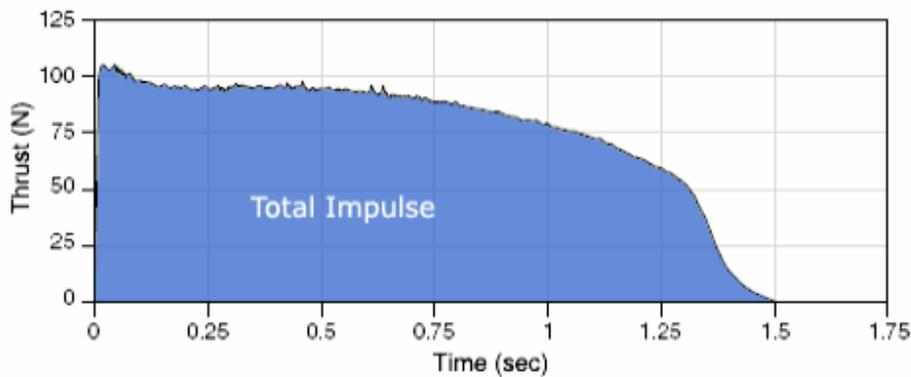
Figure 1 – A “G” Class rocket engine’s thrust/time curve. <http://thrustcurve.org/enginestats.shtml>
