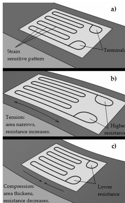
**Figure 5: A strain gauge**
