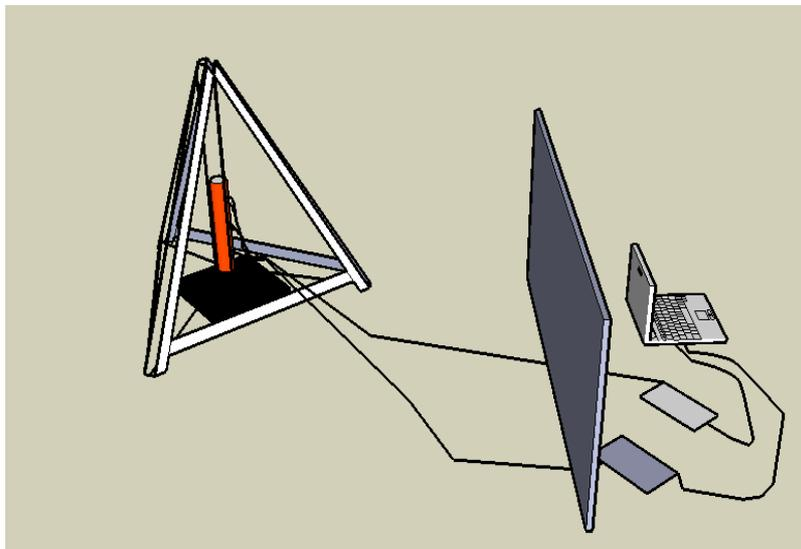
**Figure 7:** A laptop collecting data from the sensors via Labpro and a protection shield to protect the laptop from debris from a potential rocket failure.
