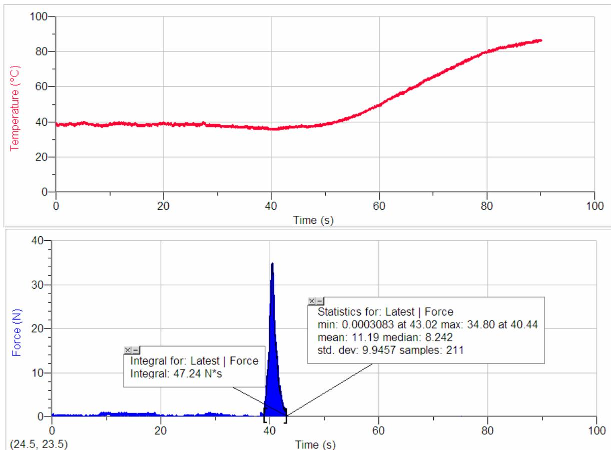
Figure 9: The engine's peak thrust was approximately 34.8 N, and the outside of the case reached approximately 86.2°C at the peak of the graph. The total impulse that this rocket produced was 47.24 N\*s.
