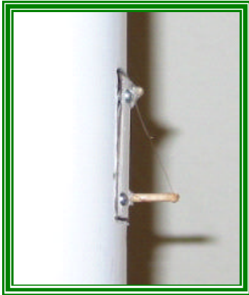
Figure 8. Rocket mounted type T thermocouple. The junction is visible near the center of the sensor.
