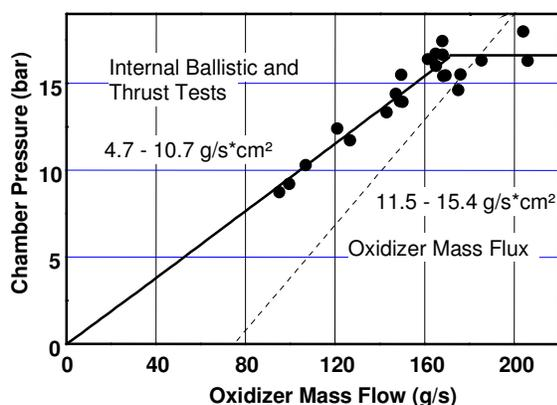
Figure 12: Chamber Pressure versus Oxidizer Mass Flow (single port grain)
