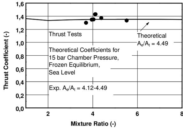
Figure 18: Experimental & Theoretical Thrust Coefficient versus Mixture Ratio
