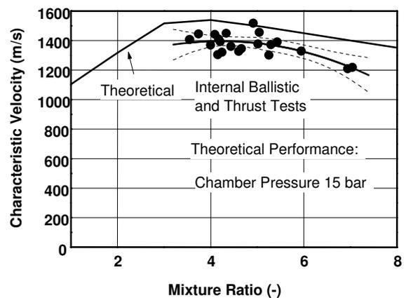
Figure 17: Experimental & Theoretical Characteristic Velocity versus Mixture Ratio
