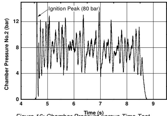
Figure 16: Chamber Pressure versus Time Test
