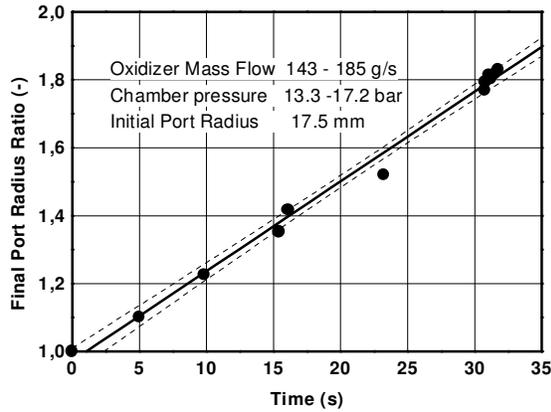
Figure 20: Final Port Radius Ratio versus Time
