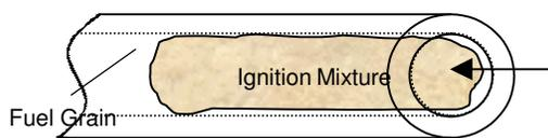
Figure 4: Application of Ignition Mixture
