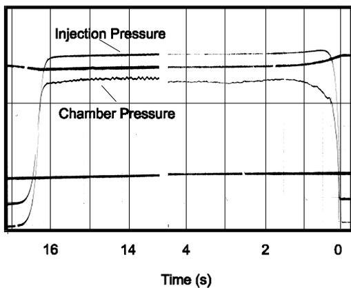
Figure 15: Typical Smooth Internal Ballistic Test
