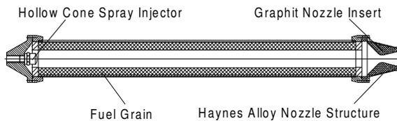
Figure 8: Configuration of Thrust Test Motor
