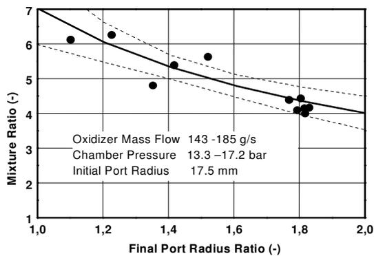
Figure 21: Mixture Ratio versus Final Port Radius Ratio
