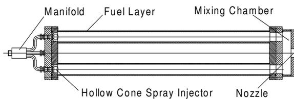
Figure 9: Configuration of Testbed Motor
