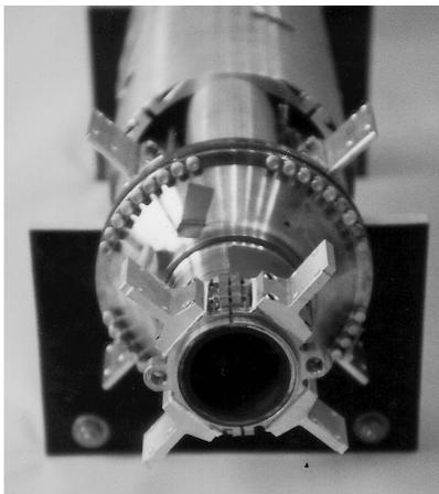
Figure 3: Nozzle Assembly of Rocket
