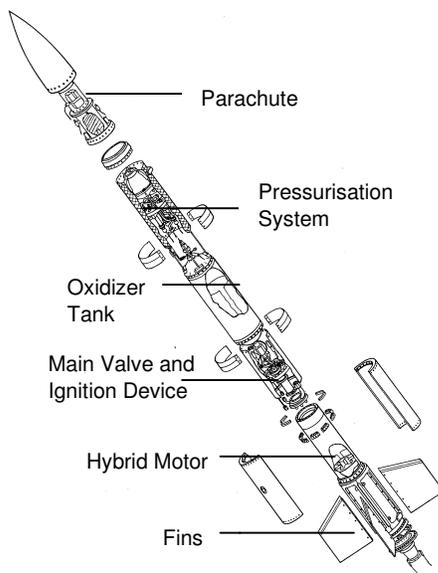
Figure 2: Final Configuration of HERA
